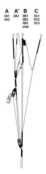
Difference not more than +/- 5mm for the length laid down in the User's Manual.
