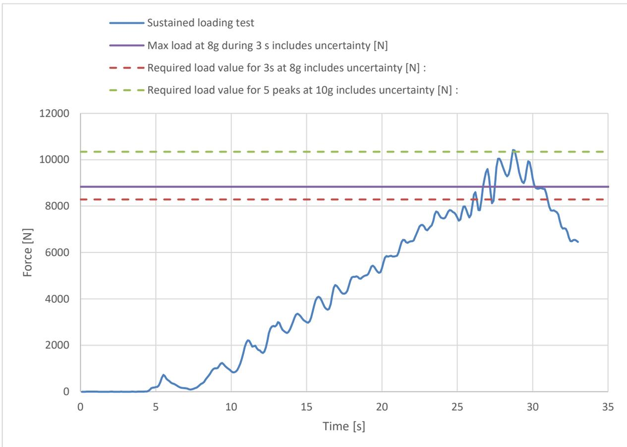
**Sustained loading test results <sup>(3)</sup>**
